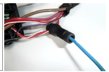
6. To properly use crimpless solder butt connectors, strip the wire insulation back and insert a wire through one side and then twist the 2 wires together. Next, center the connector on the bare wires and use a heat gun to melt the solder. Be careful with the surrounding area as the internal solder can take awhile to melt. Finally, verify the connection is solid by gently tugging.
