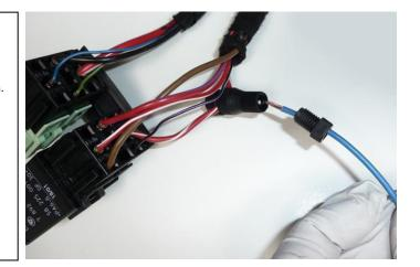
5. Screw the Posi-Tap connector together and give the wire a quick tug to make sure it seated properly.
