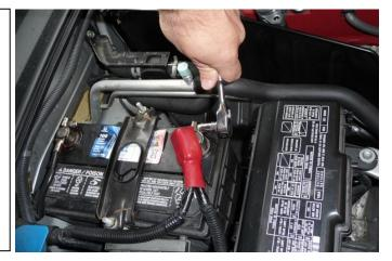
7. Connect the "GROUND" ring terminal to a clean bare metal chassis surface.
